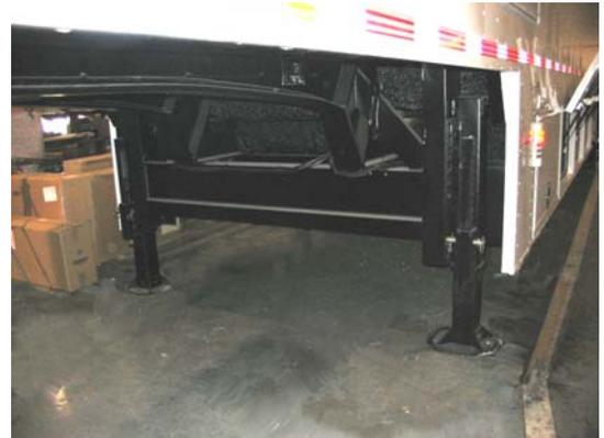
**Figure 49: Landing / Stabilizing Leg Assembly**
