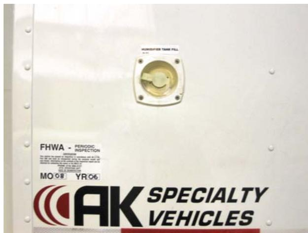
**Figure 43: Humidifier External Water Connection**
