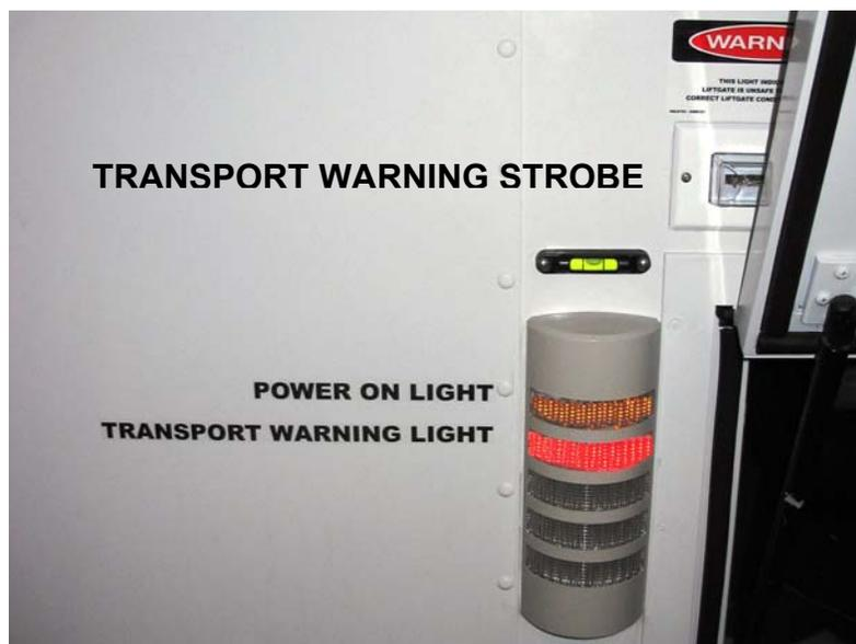
[Figure 60: Lift Transport Warning Strobe](#)
